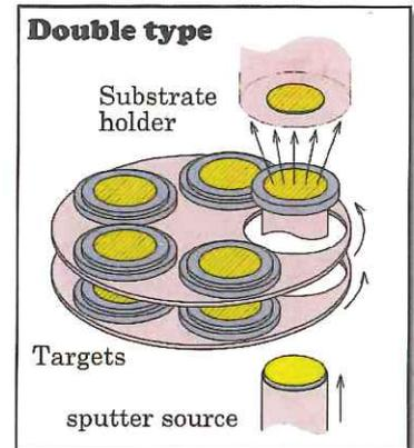
Fig.2 Structural drawing.
